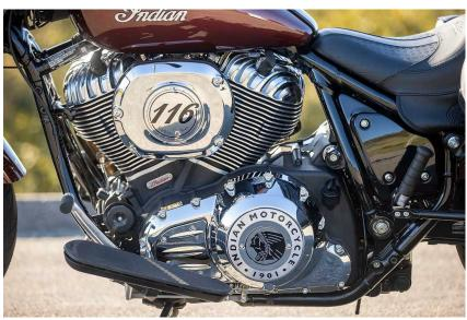
The Super Chief Limited is extra "super" thanks to the 1,890cc air-cooled V-twin Thunderstroke 116 engine, an upgrade from the Thunderstroke 111 powerplant in the base-model Super Chief. The Thunderstroke 116 is torquey down low and will happily cruise along in the 3,000 rpm range with a tolerable buzzing in the bars and the seat.
